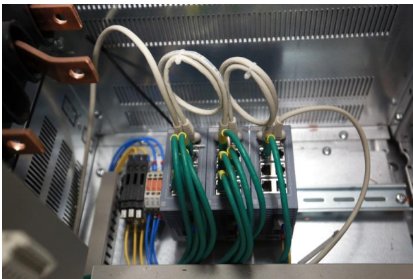
Photo 6 Customer network topology using a Ethernet switch
